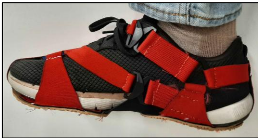
Figure 1: The instrumented shoe cover.
